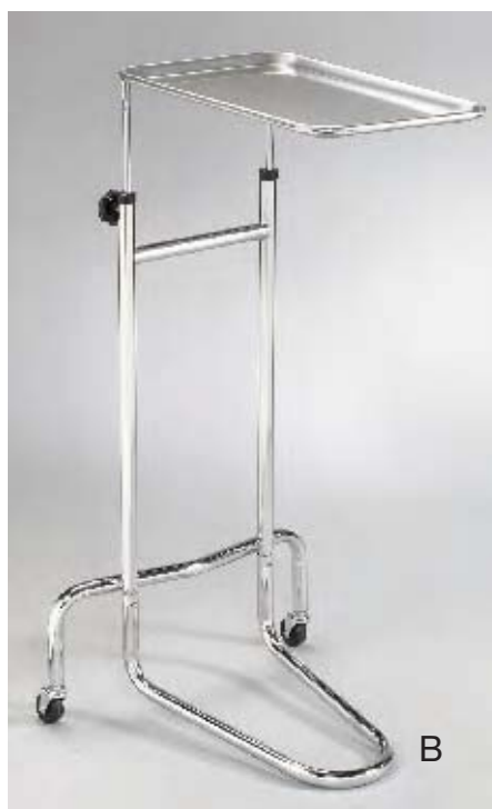
B CMA-22 Double Post Mayo Stand • Removable stainless steel tray • 2 ball bearing, rubber casters • 1" chrome plated poles and base • Easy position base • Base: 21" x 20" • Height range: 34"-54"
