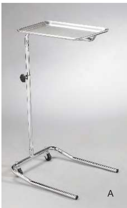
A CMA-21 Single Post Mayo Stand • Removable stainless steel tray • 2 ball bearing, rubber casters • Chrome plated poles and base • U shaped base • Base: 18" x 22" • Height range: 31"-50"
