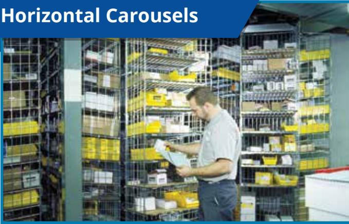
This automated storage system will make your facility more productive and space efficient. Shelves rotate horizontally to bring parts to the operator, eliminating travel time and reducing picking errors.
