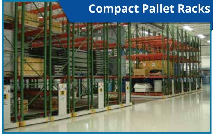
Compact pallet racks can cut your floor space in half by mobilizing rows of pallets with the push of a button, even remotely from a fork truck. Reduce floor space dedicated to pallet storage without giving up 100% accessibility.
