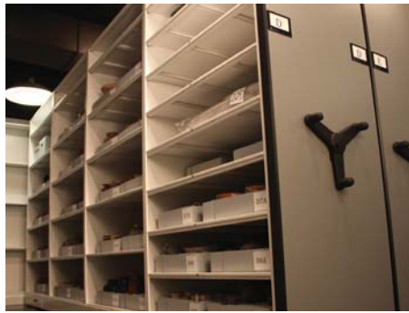
(Above) A Spacesaver high-density storage system offered the ability to store the same size collection in half the space. (Right) A study room with a camera mounted above a large conference table allows students a close-up view of valuable artifacts.
